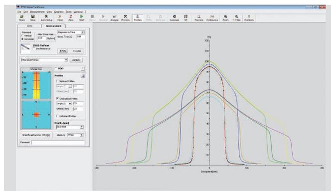
FFF beam profiles are automatically detected and evaluated following recommendations of Fogliata et al. The acquired beam data can be quickly analyzed according to international or vendor-specific protocols. A table generator makes it easy for users to automatically calculate TPR/TMR, OCR and output factors.
