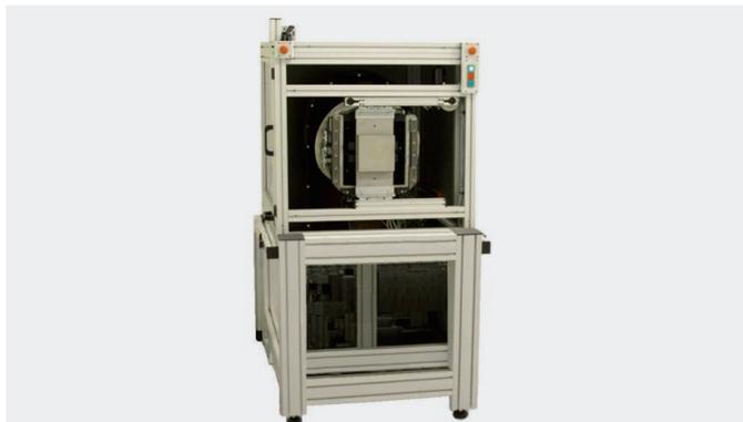
The TERABALT T-100 represents a laboratory irradiator which serves for applications where “hard” gamma radiation of  $^{60}\text{Co}$  (1.17 and 1.33 MeV) is used. Primarily, the T-100 is designed for calibration laboratory needs.
