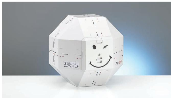
The treatment of multiple metastases with one isocenter is getting increasing clinical relevance. These non-isocentric treatment techniques require additional quality assurance. The System QA MultiMet insert is dedicated to the systematic QA of these irradiation techniques, with or without couch rotation.
