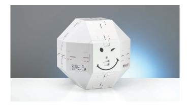
The treatment of multiple metastases with one isocenter is getting increasing clinical relevance. These non-isocentric treatment techniques require additional quality assurance. The System QA MultiMet insert is dedicated to the systematic QA of these irradiation techniques, with or without couch rotation.
