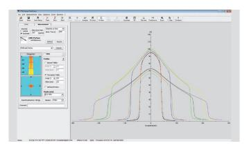
FFF beam profiles are automatically detected and evaluated following recommendations of Fogliata et al. The acquired beam data can be quickly analyzed according to international or vendor-specific protocols. A table generator makes it easy for users to automatically calculate TPR/TMR, OCR and output factors.
