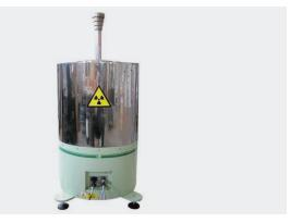
PGI-01 irradiator is primarily intended for the calibration and testing of personal dosimeters with a non-collimated source or can be used as a general panoramic source of gamma radiation. For this purpose, PGI-01 has to be fitted with a suitable radionuclide.
