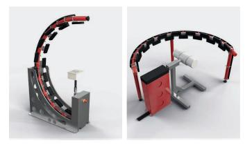
Up to 18 chambers can be mechanically arranged on a semicircular arch of 1 m radius according to IEC. The X-ray tube is positioned on a rotatable table and – while the table is continuously rotated – the XLS leakage system monitors the dose rate of all detectors and records the radiation levels of the entire hemisphere around the X-ray tube. The rotatable table and the chamber fixation parts are neither part of the XLS chambers nor the XLS X-ray leakage system.
