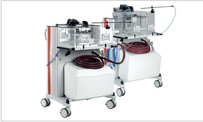
**BEAMSCAN® MR** is a complete solution for the commissioning and QA of MR linacs – from automatic beam data acquisition and processing to data analysis and protocol-based documentation. The system is dedicated for use with MR linacs up to 1.5 T.
