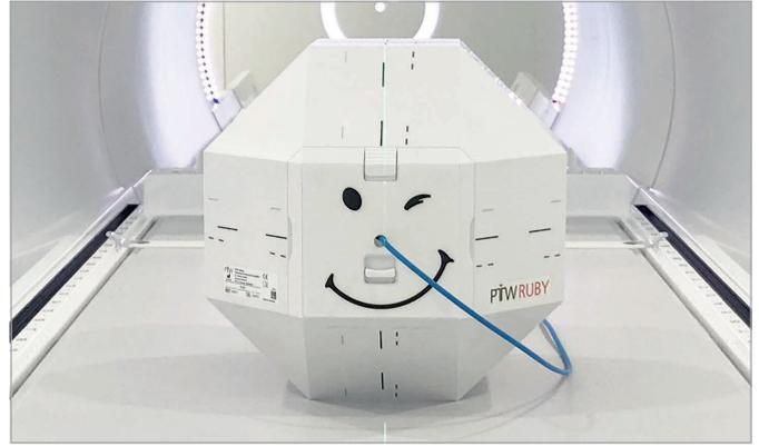
The System QA insert features MR visibility in T1 and T2 at 1.5 T and allows the positioning of an MR compatible detector in the center of RUBY. End-to-end QA can be performed using the adapt-to-position or the adapt-to-shape workflow.
