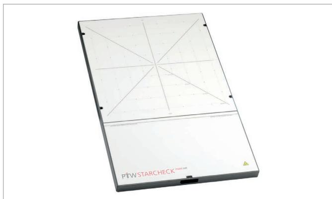
The **STARCHECK® maxi MR** is a precise and reliable tool for fast measurements in radiation therapy beams. A typical application of this array detector is quality control. The ionization chambers feature an excellent relative response stability, eliminating the need for frequent recalibration. A full set of 4 profiles is measured every 400 ms (or one profile every 100 ms).
