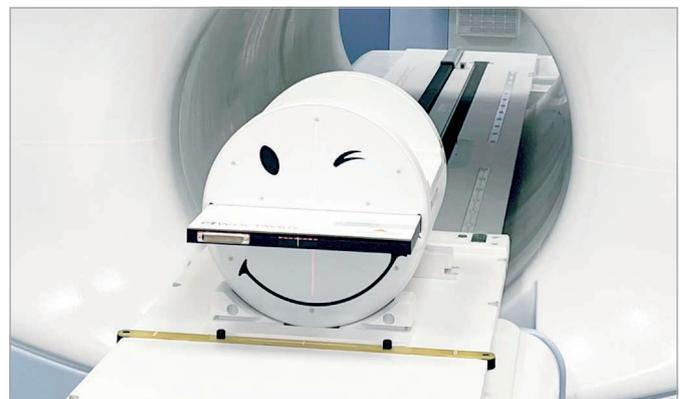
The **OCTAVIUS Detector 1600 MR** is the MR Conditional version of the OCTAVIUS Detector 1600 SRS. It is a liquid-filled 2D array detector. The very small detector size of only 2.3 mm x 2.3 mm x 0.5 mm makes this array detector ideally suited for small field dosimetry.
