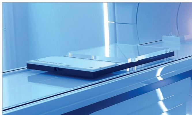
The excellent spatial resolution of only 3 mm ensures precise measurements even in penumbra regions. The scanning lengths covered by the detectors are 40 cm along the principal axes and 56.5 cm along the diagonals. This makes STARCHECK maxi MR an easy-to-use tool for your daily QA tasks.
