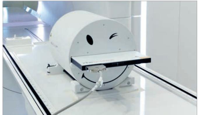
The OCTAVIUS 4D MR can be used with the MR Conditional array detectors **OCTAVIUS Detector 1600 MR** and **OCTAVIUS Detector 1500 MR**.
