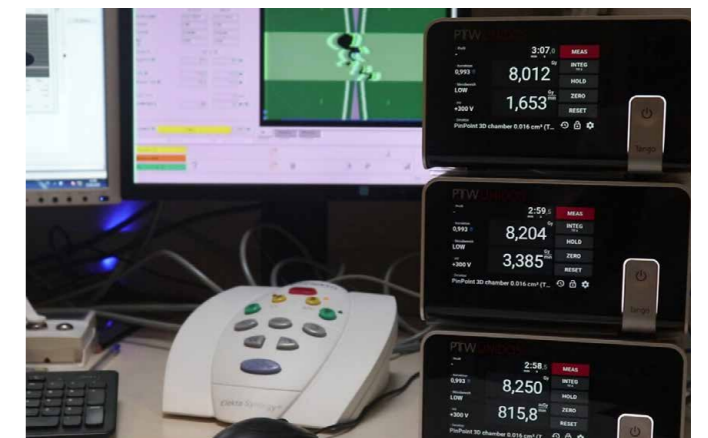
Figure 21: Simultaneous dose measurement in the System QA MultiMet insert using three PinPoint 3D ionization chambers and three UNIDOS Tango systems
