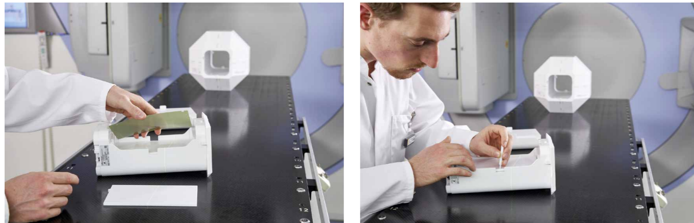
Figure 10: Patient QA film insert allows the use of a 17 cm x 9 cm sized radiochromic film. A marking plate is used to mark the film relative to the CT markers in the phantom.
