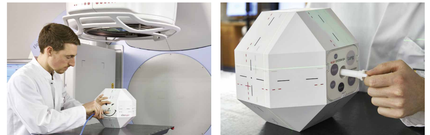
Figure 17: The detector holder corresponding to the detector is screwed into the insert on the back and the detector is inserted into the insert from the front. This method ensures an exact positioning of the detector in the phantom center in relation to the CT markers.
