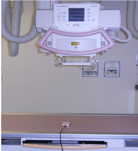
Picture 17: NOMEX Multimeter under the tube and within the radiation field
