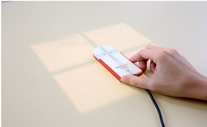
Picture 4: Positioning the NOMEX Multimeter within the radiation field in digital radiography
