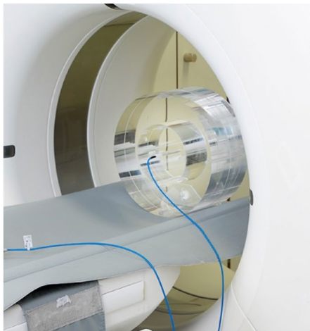
Picture 22: Adjust the CT body phantom and insert the CT chamber
