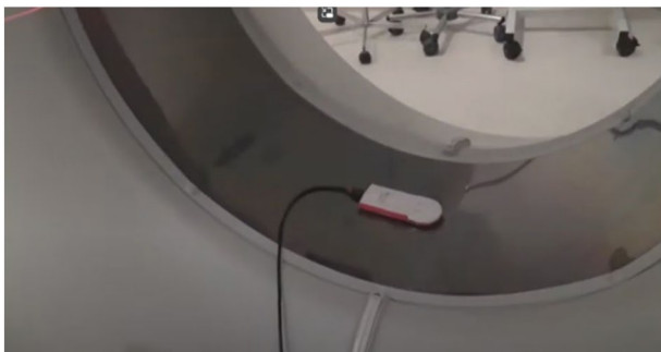
Picture 24: NOMEX Multimeter setup with CT
