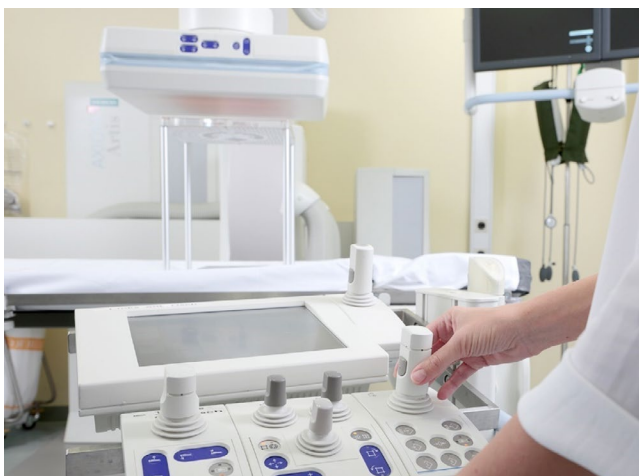
Picture 1: Adjustment of the NORMI RAD/FLU phantom at a digital fluoroscopy unit using a dynamic flat panel
