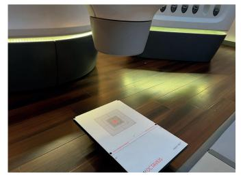
Figure 11: Measurement setup for the Laser and Radiation Coincidence check
