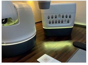
Figure 12: Measurement setup for the Laser and Radiation Coincidence check with the double height
