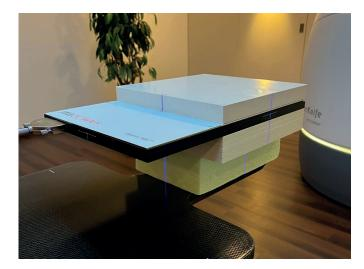
Figure 4: Measurement setup for patient-specific QA
