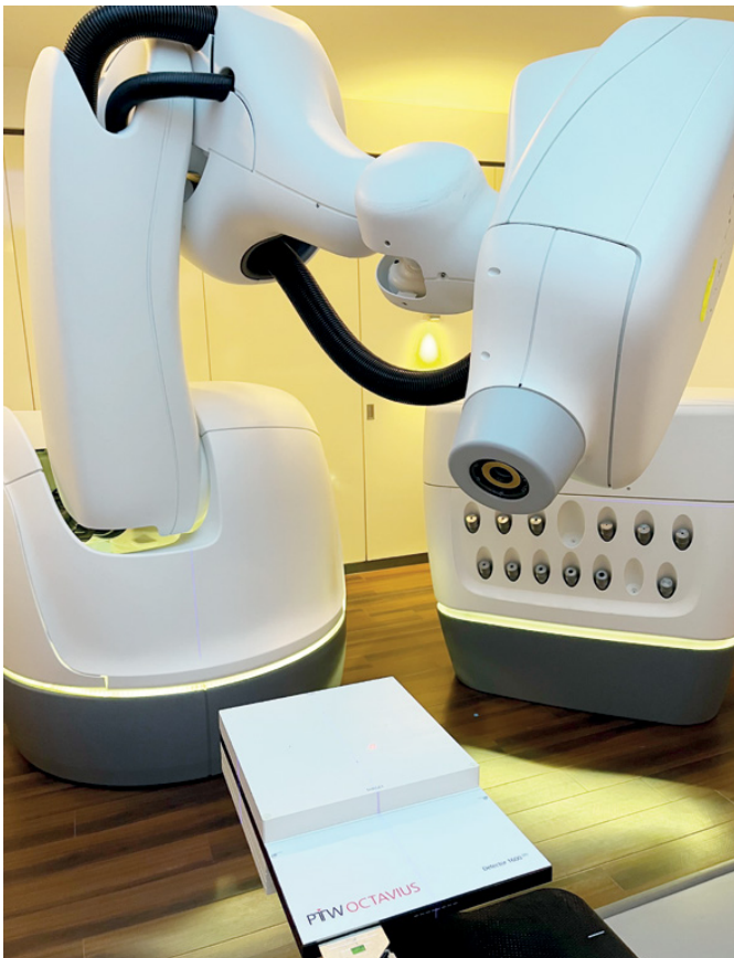
Figure 1. Fast and simple workflow: CyberKnife® QA with OCTAVIUS Detector 1600 SRS.
