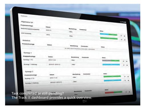
When creating tasks in a protocol template, an entry must always be assigned from the list of data types. Data types of PTW measuring devices are automatically recognized by Track-it during the first data transfer and automatically added to the database. However, if data from third-party devices or individual data types are used for measurement tasks that are not yet available in the system, it is important to add the new data types before creating the protocol templates.
