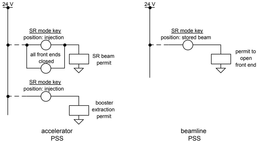
Figure 8: Logic used until now in the machine and beamline personal safety systems associated with the storage ring injection.
