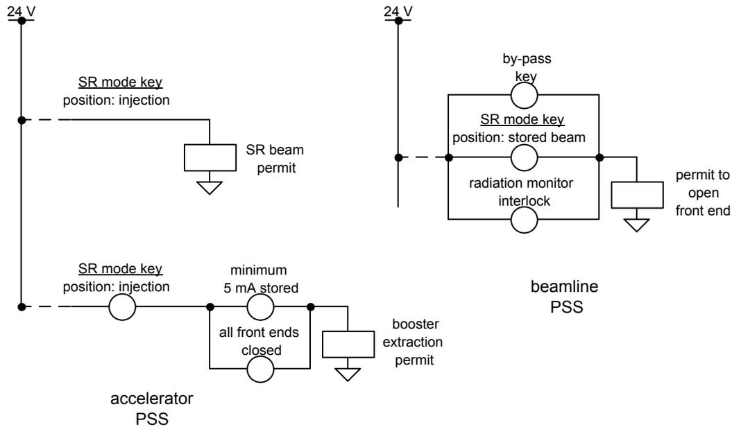
Figure 9: Logic used to implement injection with front ends open in the machine and beamline personal safety systems.
