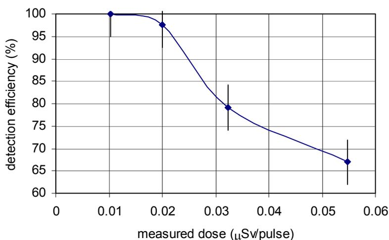
Figure 3: Experimentally determined efficiency curve for measuring pulsed radiation with the Apfel REMbrandt neutron monitor.
