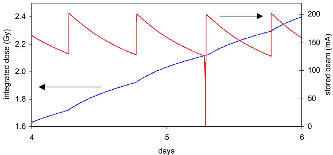
Figure 5: Integrated on-axis dose inside the ID6 optics hutch during 2 days of hybrid mode operation.
