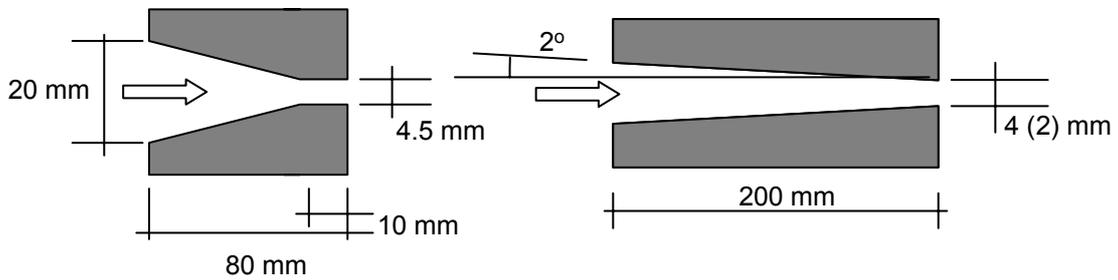
Figure 2: 4.5 mm diameter copper aperture in undulator beamlines (left). In the new high power front ends, a similar rectangular  $4 \times 4$  mm<sup>2</sup> (or  $4 \times 2$  mm<sup>2</sup>) copper aperture is installed (right).
