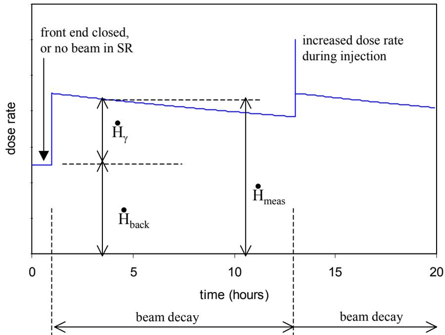
Figure 7: Typical measured dose rate pattern.
