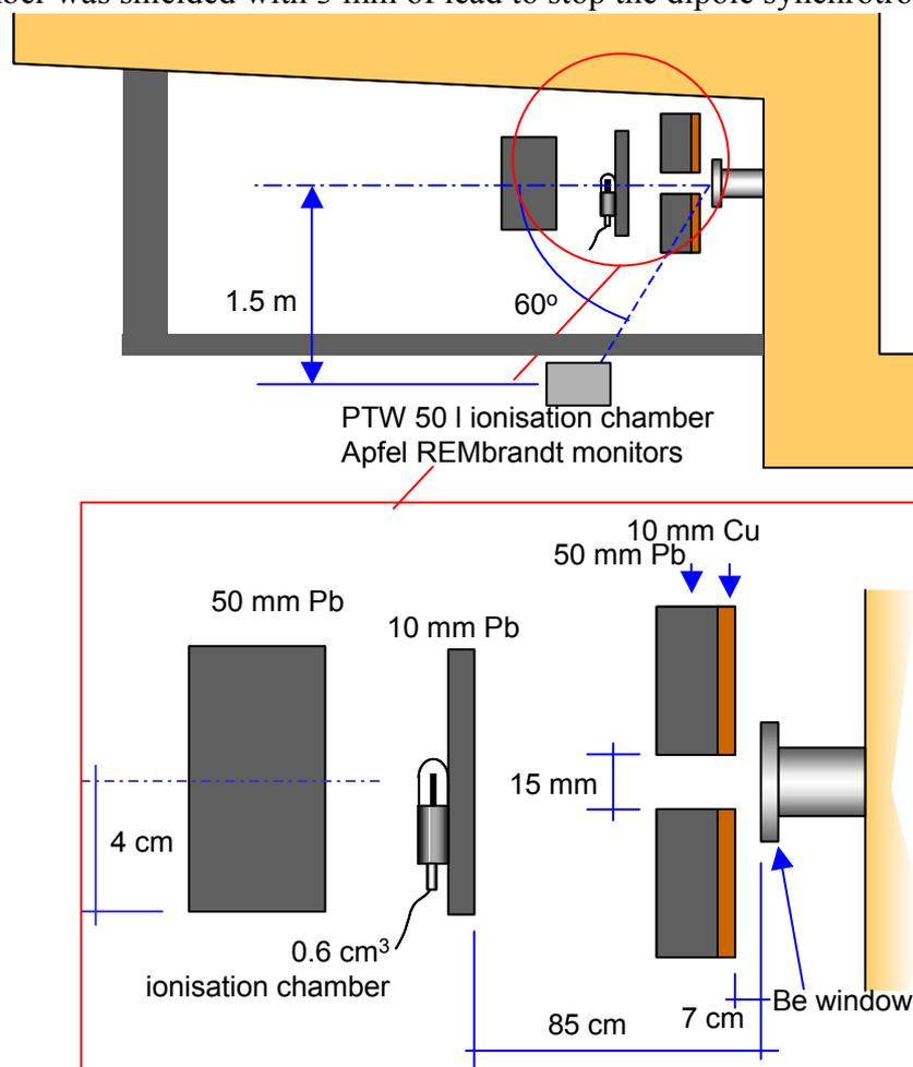
Figure 1: Experimental set-up used for the radiation measurements
