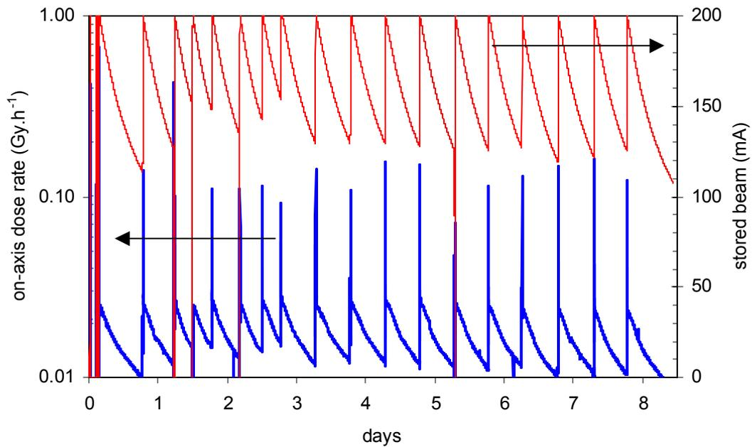
Figure 4: Measured on-axis dose-rates inside the ID6 optics hutch during 8 days of hybrid mode operation.
